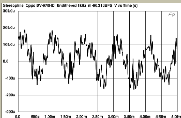
Fig.5 Oppo DV-970HD, waveform of undithered 1kHz sinewave at -90.31dBFS, 16-bit data.
