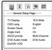
2. Press the LEFT/RIGHT ARROW buttons to select the setup page. There are 5 pages: General Setup, Speaker Setup, Audio Setup, Video Setup, and Preference. Press the SELECT button to enter the selected setup page. The Preference page can only be accessed when playback is completely stopped, or when there is no disc in the player.
